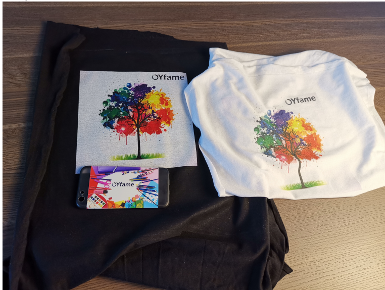
5 Heat press machine 170° degrees 60 seconds
